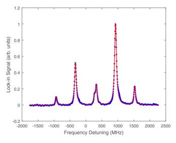
FIG. 4. A sample HFS reference signal measured via IR light transmitted through a supplementary indium vapor cell. The solid line is a curve fit using a sum of six Lorentzians. The six peaks include two hyperfine features, each with two sidebands. The central two sidebands are partially overlapped but can be resolved in the fitting procedure. This signal is used for frequency calibration and referencing as well as to measure the  $6p_{1/2}$  hyperfine splitting, as described in the text.
