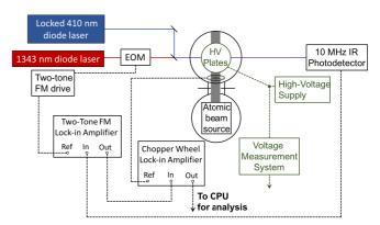
FIG. 5. A schematic diagram detailing the atomic-beam unit setup, including the detection electronics using two successive lock-in amplifiers.
