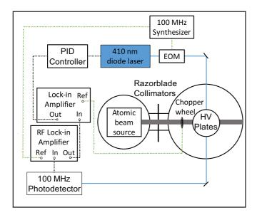
FIG. 2. Schematic diagram showing the optical and signal processing arrangement for the atomic-beam-based laser locking scheme.
