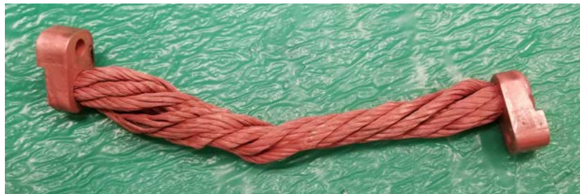
Figure B.7: The oxide formed during the welding process has been removed with an acid (typically Citranox) bath. This heat link is ready for installation.
