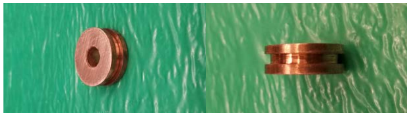
Figure B.3: Copper bobbin used for a wire heat sink. Center hole is a 10-32 screw hole, outer diameter is non-critical. The channel cut in the side makes it easy to wrap and epoxy the wire.
