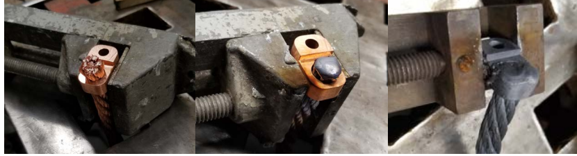
Figure B.6: (left) Copper lug arranged to be welded. The connector is slightly above the surface of the vise so that the welding arc does not form to the vice. (center) Step 1, the copper braid has been melted into a solid mass. (right) The solid copper braid has been melted into the surface of the copper connector.
