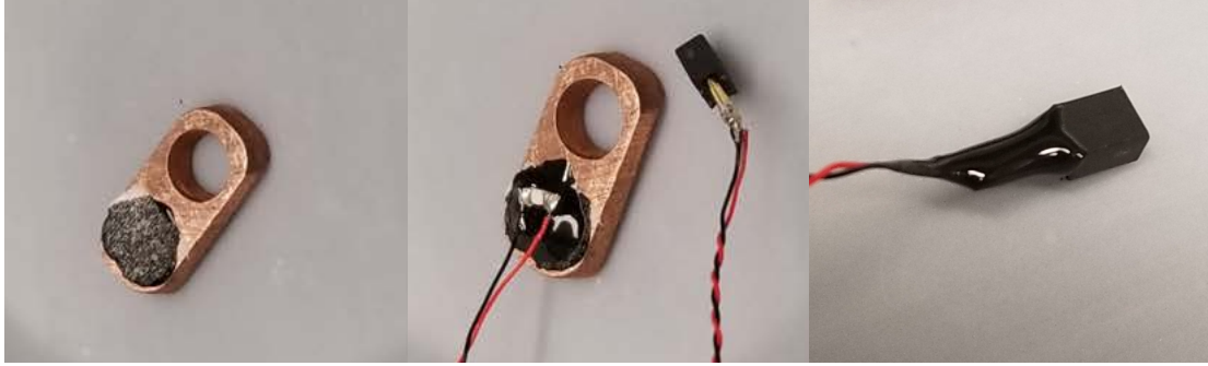
Figure B.2: (left) Copper mount with epoxy and electrical insulator. (center) The resistor is fully encased in epoxy. (right) The electrical connection has been strain relieved with epoxy.
