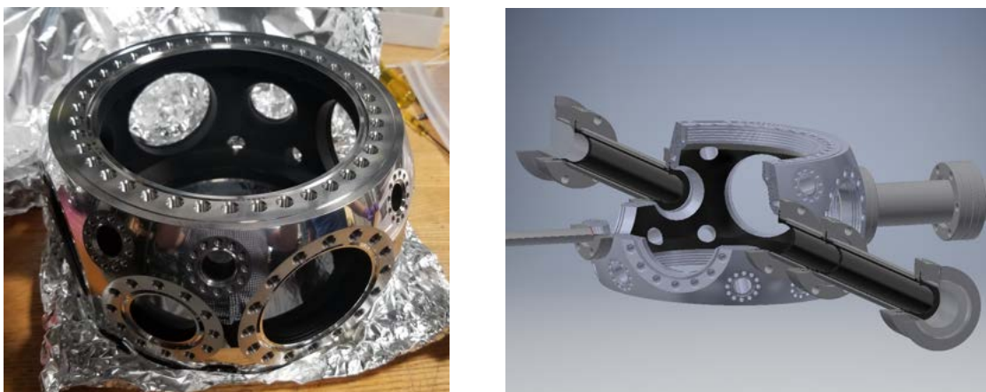
Figure 8.3: (left) Image of the Acktar Magic black coated vacuum chamber. (right) Machine drawing of the blackened vacuum chamber with blackened copper tubes and razor edge baffles.
