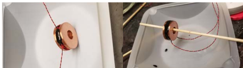
Figure B.4: Applying Stycast epoxy to a wire heat sink. (left) apply a small dot of epoxy to secure the wire. The ends of the wire are tensioned with tape. (right) The channel in the bobbin is flooded with epoxy to ensure a large surface area for thermal contact. The bobbin is elevated to ensure that the Stycast does not adhere to the working surface.
