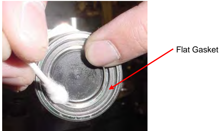
Figure B-2: Cleaning the male Aeroquip®
