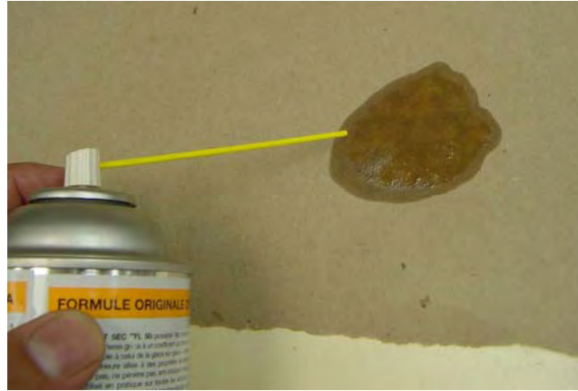
Figure B-4: Typical amount of lubricant
