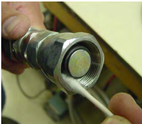
Figure B-1: Cleaning the female Aeroquip
