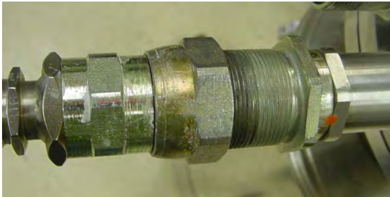
Figure B-3: Female to male connection, hand tightened
