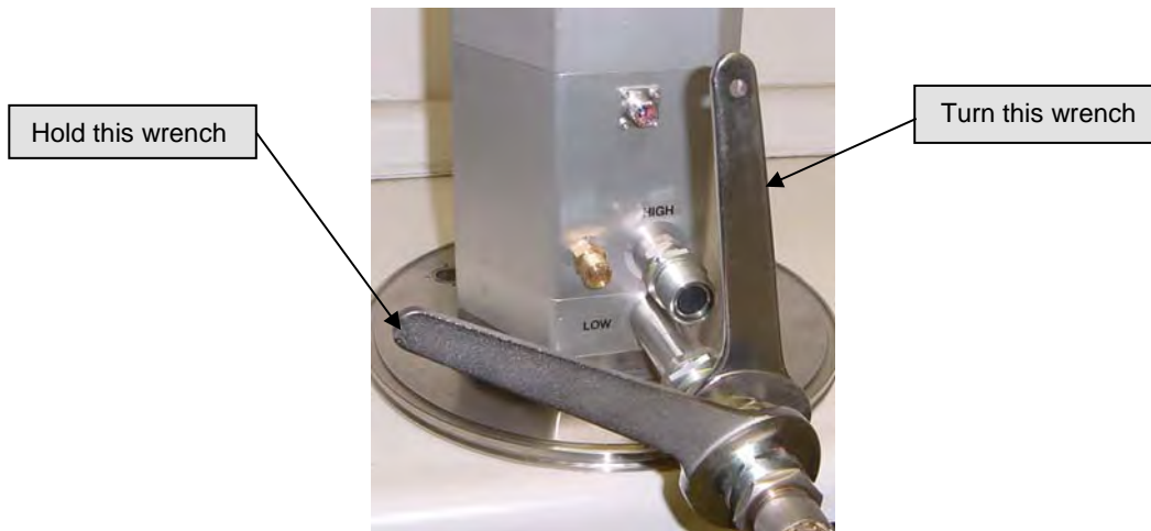
Figure 6-4: Connecting the low-pressure flex line to the low-pressure port on a cold head
