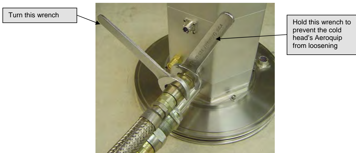
Figure 7-2: Disconnecting flex lines from a cold head
