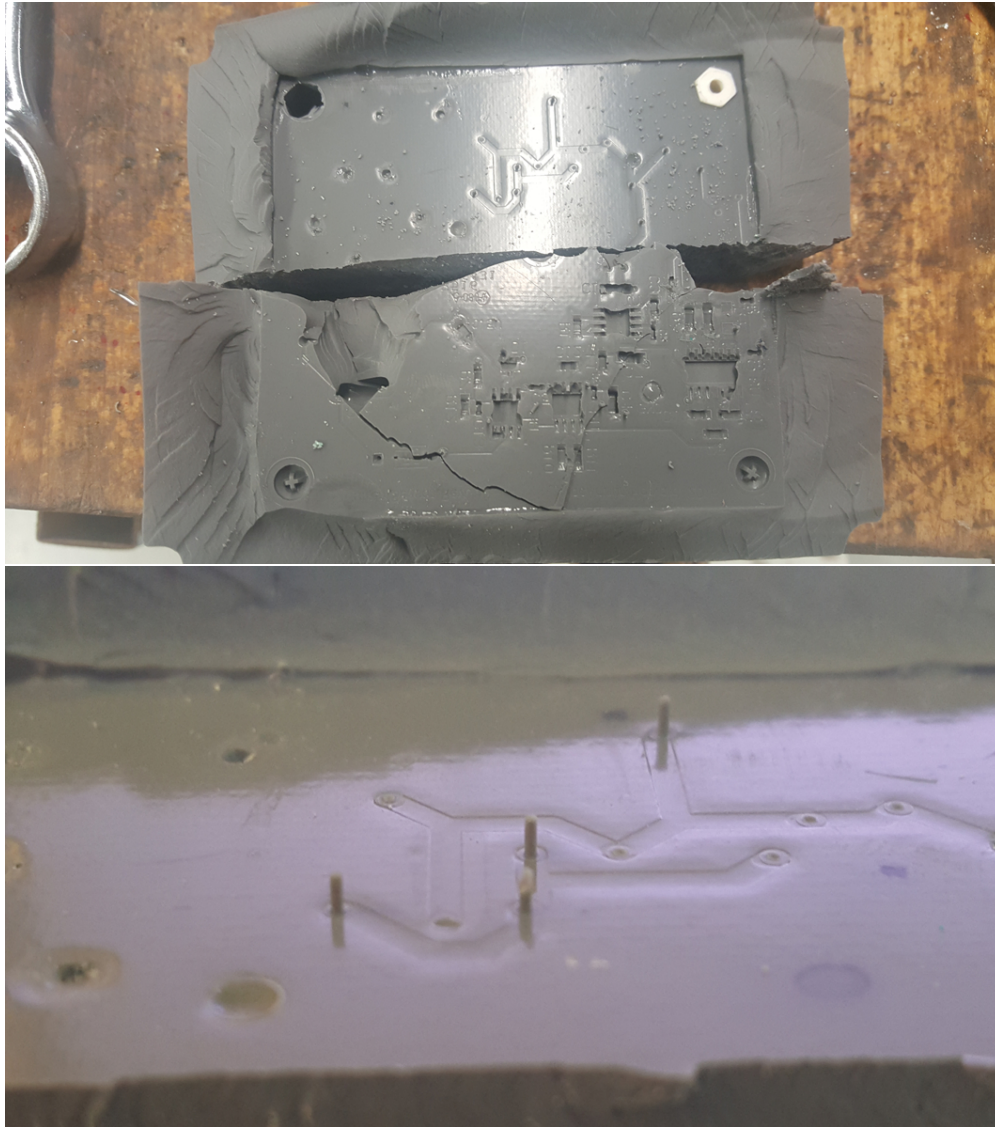
Figure 12: Pieces of silicone that were used to pot the ammeter.
