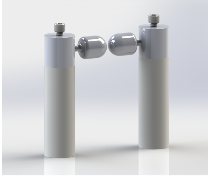
Figure 3: Spark gap design. Spherized aluminium electrodes have an external tap so that they screw into aluminium cylinders. These cylinders attach via set screw to nylon cylinders. On top of the aluminium cylinders are 1/4-20 threads to make connections via spade connectors. The bottom of the nylon cylinders are threaded such that you can screw in a pedestal base so that they may be clamped to a breadboard. The separation of the electrodes can be finely adjusted by screwing the electrodes in or out.
